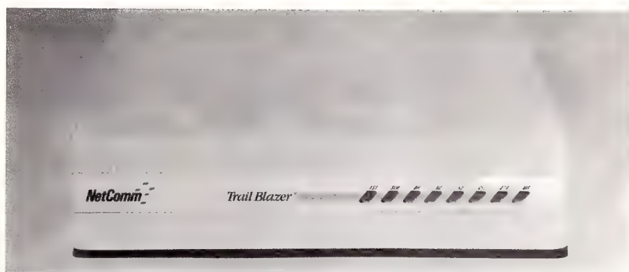
Figure 1. Perhaps one of the best-kept secrets about the Trailblazer is the fact it is also a fully-functional, Hayes compatible multi-standard modem which can talk at our 1200 and 2400 bits per second, as well as the US Bell 300 and 1200 bits per second standards. It doesn't do V21 (our 300 bits per second) or V23 (1200/75), but they are almost totally irrelevant these days anyway.
