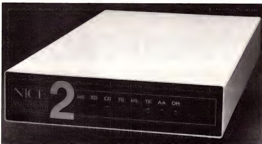
Figure 5. The Nice Modem 2 offers a dialing directory and ring-back security.
