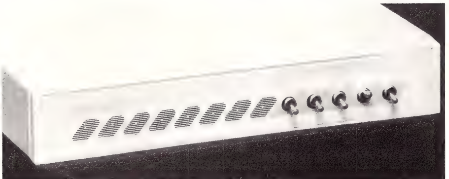
Figure 4. The NetComm 1234A has been superseded by the 1234SA (shown above) which supports synchronous transmission.
